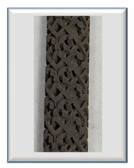
Catalytic static mixers are a novel immobilized catalyst system, based on 3D printed mixer scaffolds containing a catalytic active layer. A variety of different active catalysts can be deposited on the metal mixer, allowing employment in many different classes of chemical reactions, such as hydrogenations, oxidations, C-C couplings and many more. Pt mass is ~1500mg/Mixer. Mixer volume 4849mm<sup>3</sup>.
