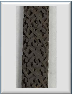
Catalytic static mixers are a novel immobilized catalyst system, based on 3D printed mixer scaffolds containing a catalytic active layer. A variety of different active catalysts can be deposited on the metal mixer, allowing employment in many different classes of chemical reactions, such as hydrogenations, oxidations, C-C couplings and many more.
